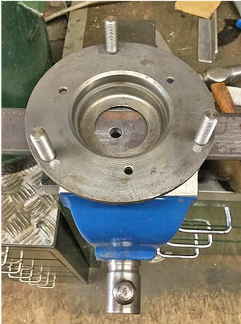
You should now have a perfectly flat undamaged surface on the carrier with all rivets flush on three new studs.
