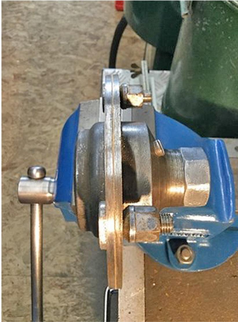
When assembled with the hub outer and a 0.012 paper gasket should have no gaps between the studs to let oil leak out into the brakes.
