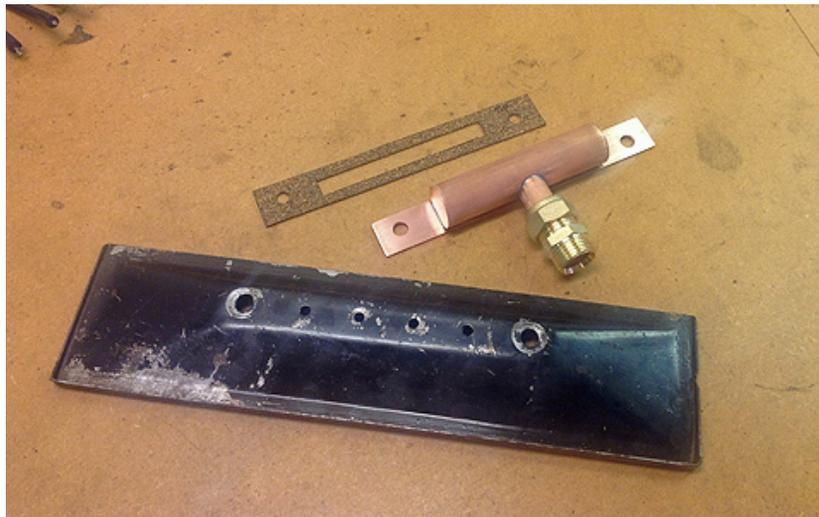
I have taken his idea and rather ploddingly built a similar device out of copper sheet and copper tubing, 15mm and 22mm plus a brass compression fitting connector.
