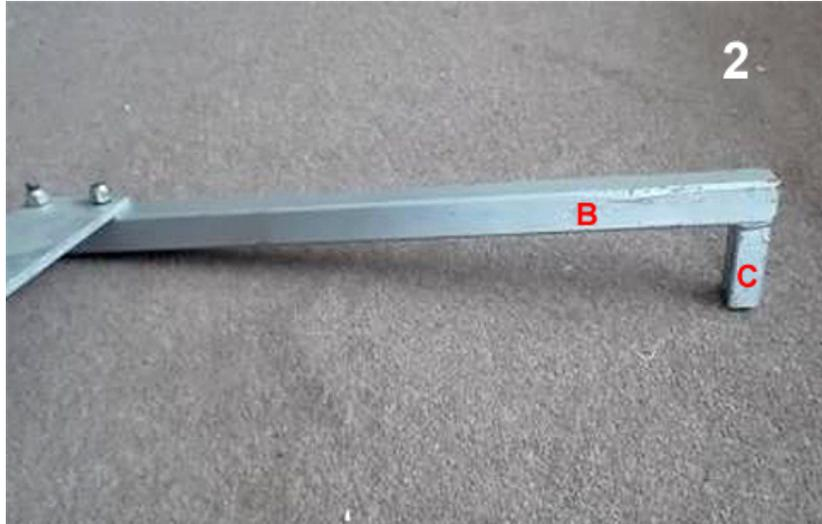
The tow bar works very well as it self-levels. With the car at the bottom of the ramps and the winch attached the tow bar swings upwards and swings downwards as the car nears the trailer bed. I leave the tow bar attached to the winch when the car is on the trailer as added security as the side arms cannot jump out from behind the axle until one side is unbolted. The other major benefit is that it pulls the car in a straight line.
