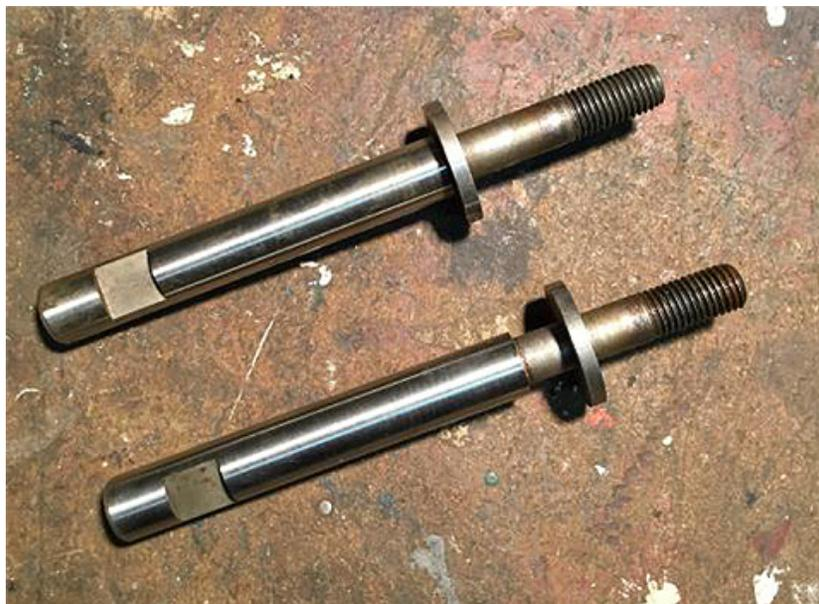
Close examination of the area where the flange diameter reduces to the pin diameter, and using an engineer's magnifying glass I was surprised to see that it appeared that the flange was in fact a thick washer!
