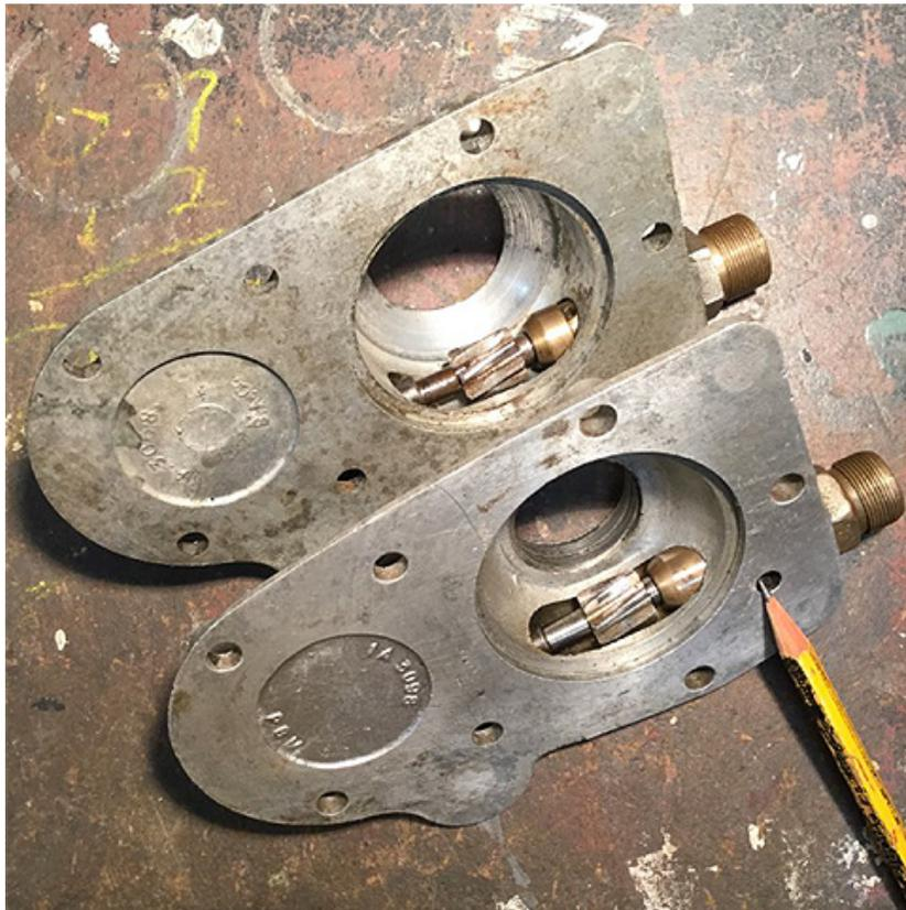
You can see how the oil gets to the speedo drive spindle in the undrilled felt seal and scroll type covers in this photo.
