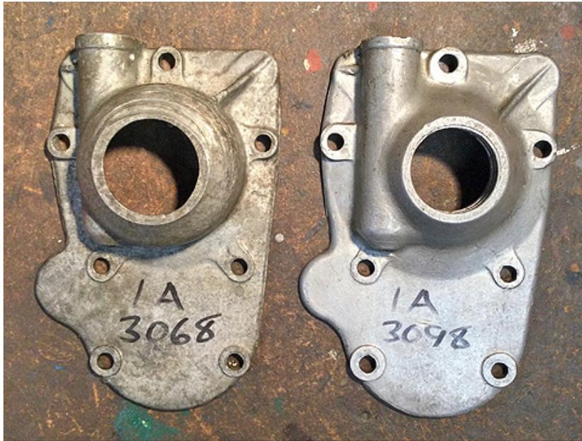
Original felt cover (left) and Scroll type cover (right)
