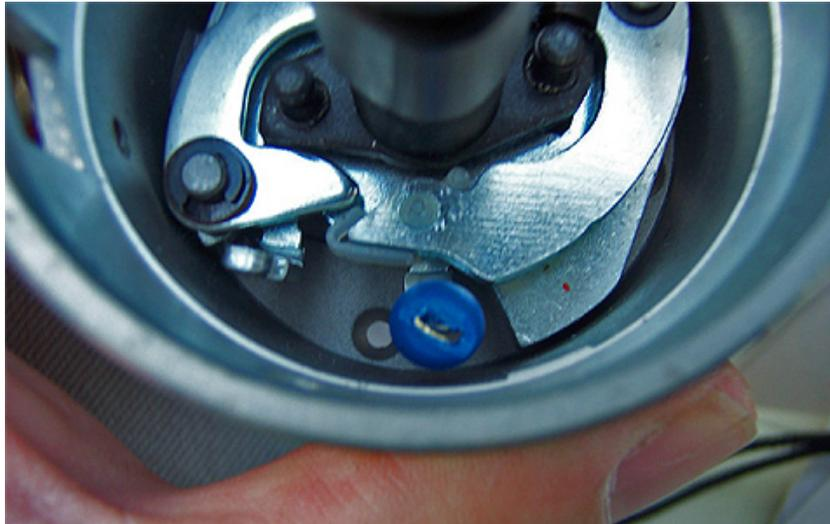
Distributor showing Geoff's mod crimped in place.
