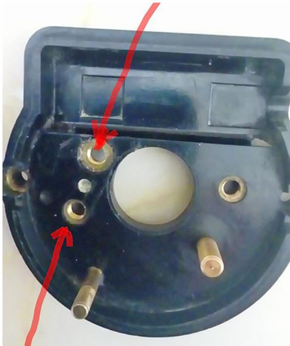
The two arrows indicate the earth return points for the Condenser and C/B, also they indicate where a temporary earth feed can be attached.
