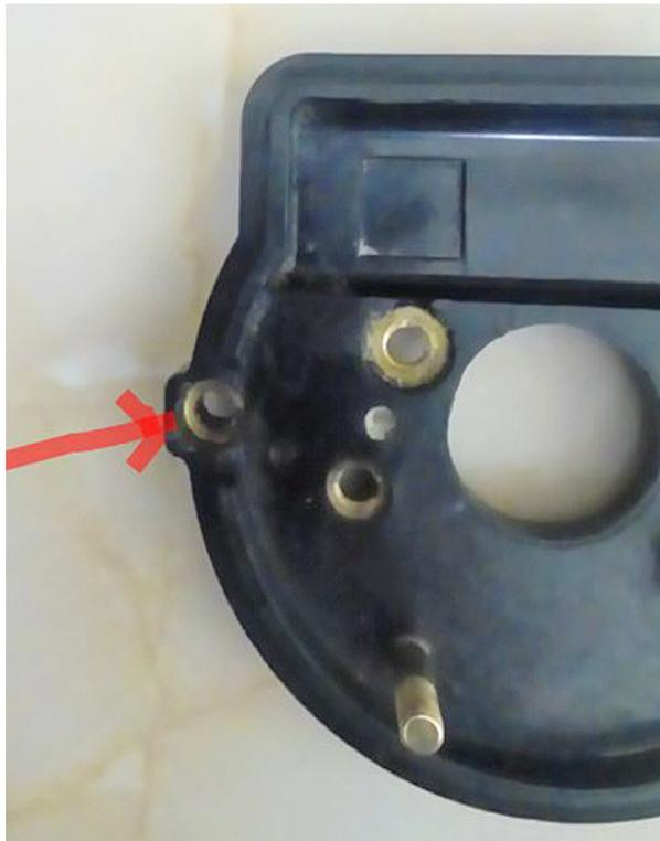
The brass washer indicated by the arrow is the return earth pick up point, this in turn is laminated via the Bakelite base plate to supply an earth return to the Condenser and C/B points.
