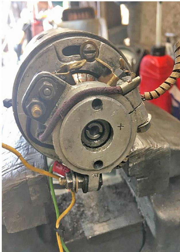
This explained the reason for having slotted holes for the attachment of the brush carrier, a fact that I did not appreciate when taking the dynamo apart. By turning the brush carrier while testing the dynamo by driving it with an electric drill the output suddenly increased and blew my 12 volt test light. It also still worked after a rest as the small amount of residual magnetism in the correct place was enough to start up the charging process.
