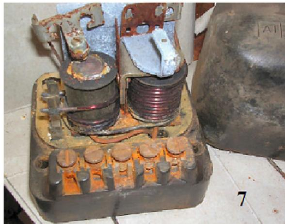
The control box I use for the conversion, is a Lucas RB 106 as in Pictures 6 & 7. These units are easily obtained from auto jumbles and Ebay. I prefer the early type that uses screw connectors. If all you can find are the later type with blade connectors these will work fine but do not look as good. Generally the RB 106 is very robust and does not give problems. However you need to remove the cover to examine the inside as there can be problems
