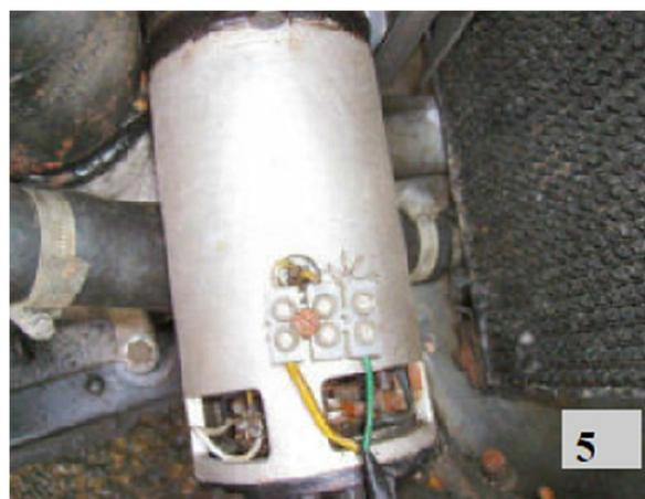
In Picture 5, I have used a three terminal connector block to replace the original two terminal standard fitting. The left terminal connects the yellow "D" lead from the control box to the dynamo "D" internal lead. The right terminal connects the green "F" lead from the control box to the extra resistance. The centre terminal connects the extra resistance to dynamo field internal cable.
