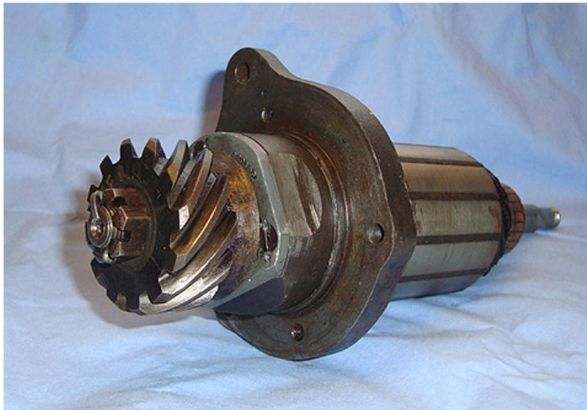
As there is plenty of metal in this grooved cover it is a fairly straight forward job to take off metal between the bottom of the groove and the end of the alloy plate. The picture shows a typical result of initial attack with an angle grinder finished off with a bit of judicious filing.
