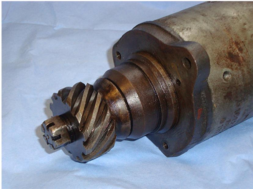
The Austin factory must have realised the pain caused by the groove and later dynamos had a conical end, as shown in the second photo, which cleared the bolt.
