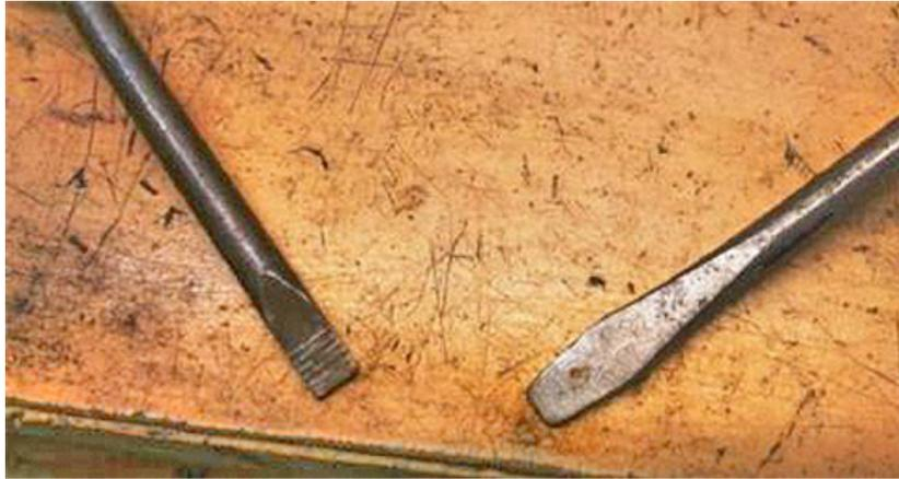
Fig 4 - The correct screwdriver is on the left. Using the one on the right will damage the main jet thread.
