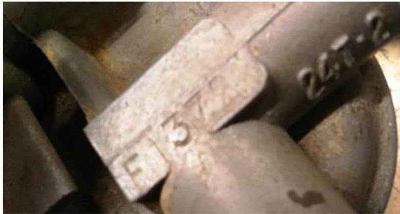
Fig 2 - Zenith type number "F1372" denotes this carburettor was built to be fitted to an Austin 7
