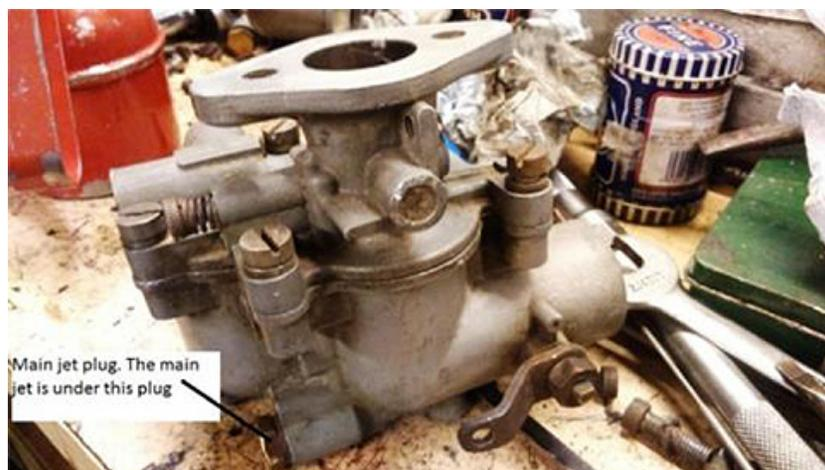
Fig 3 - Location of the main jet cover plug.
