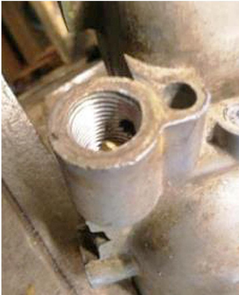
Fig 6 - Main jet thread. The main jet can be glimpsed at the bottom of the thread.
