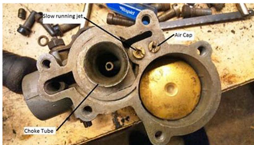
Fig 5 - Lower assembly, showing layout of jets etc.
