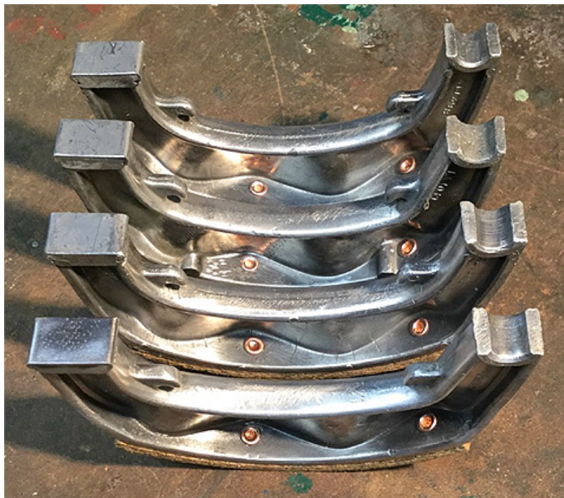
Perfect rivets and new end plates yet to be drilled and screwed.
