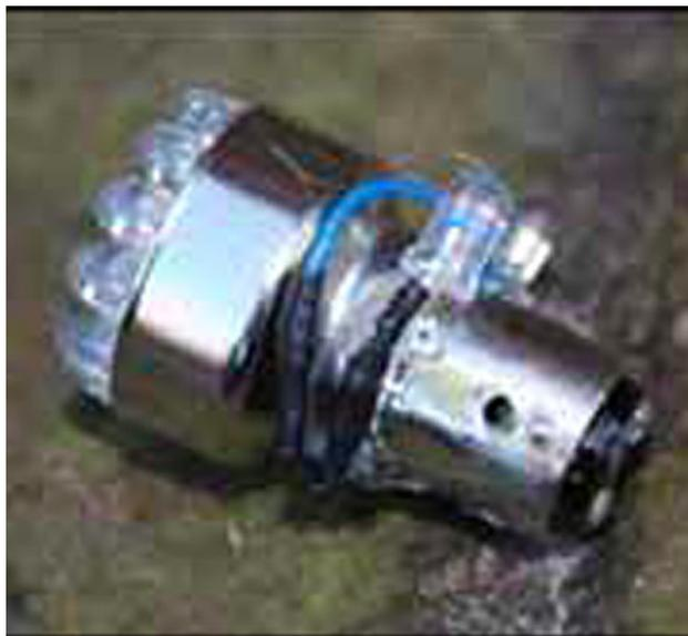
Bulb showing white LEDs added to the side and the black spot where the extra pin had been. Small resisters are inside the black heat shrink tubing.
