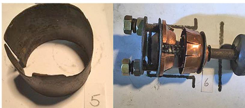
If your switch contact is like the one on the right of pic3 leave as an assembly on the button shaft and give it a good clean to bright copper. If it's badly out of
