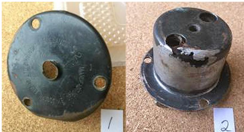
The main issue to look for is the thin brass switch cover plate wears (pic1) this results in the copper contacts of the switch not meeting squarely. The switch button copper contact becomes damaged giving a poor electrical connection with possible overheating or even a short circuit. Picture 2 shows one that has had this event and melted a hole in the steel switch body !
