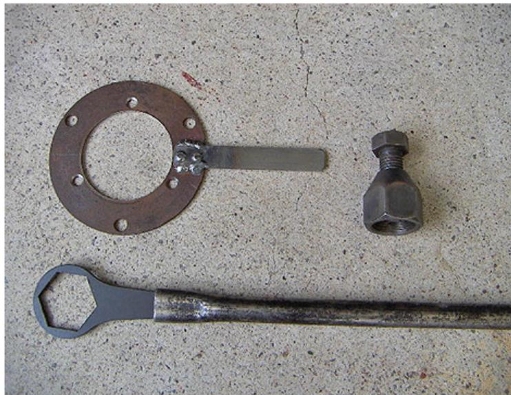
Tools for the job: Austin Hub puller (far right), home made spanner for the flat nut (bottom) and a homemade tool for holding the hub still when tightening the half shaft nut (top).
