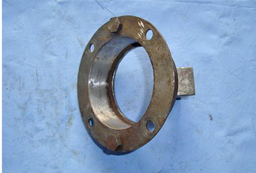
Tool B (made from a scrap housing)
