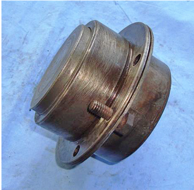
Tool A pushes outer race into tool B which is bolted to the good housing
