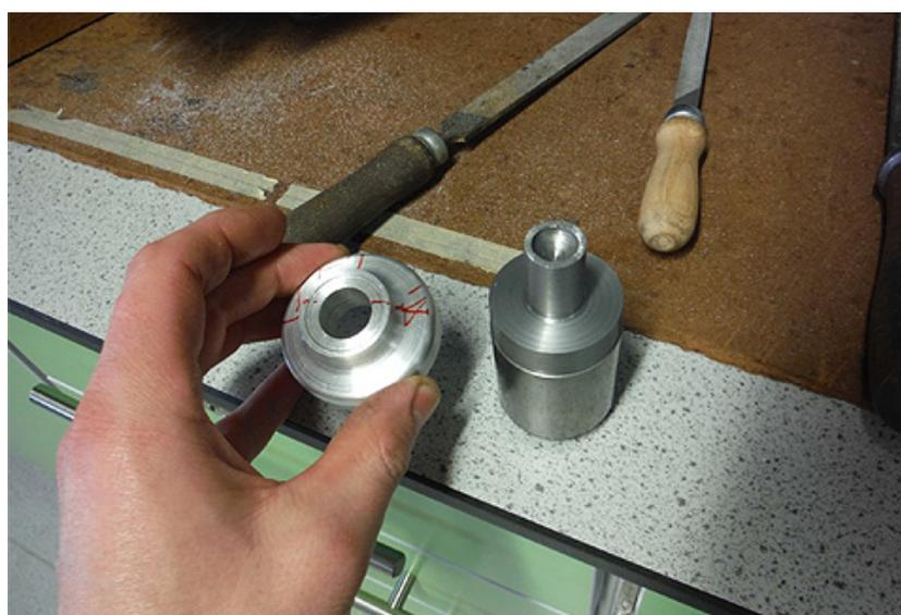
Turned part ready to cut (with steel alignment too on bench)
