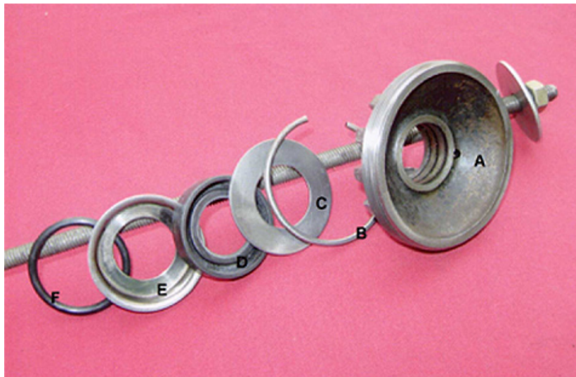
A. Adjuster B. Spring Ring C. Washer D. Oil Seal E. Seal Cup F. 'O' Ring
